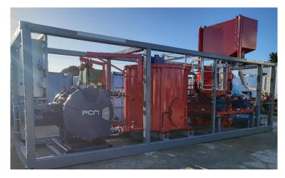
Picture shows our recently built 2 m<sup>3</sup> continuous fully computerized mixing unit which can be fed by 3 x 30-ton vertical silos holding 3 separate powders or 1 x 45ton horizonal silo holding pre-blended material (40 m<sup>3</sup>/hour of cement grout or 60+ m<sup>3</sup>/hour of liquid B/C/GGBFS grout) having 2 x duplex 100 peristaltic pumps to discharge the material. Material is recorded on a print out for each batch throughout the day.
